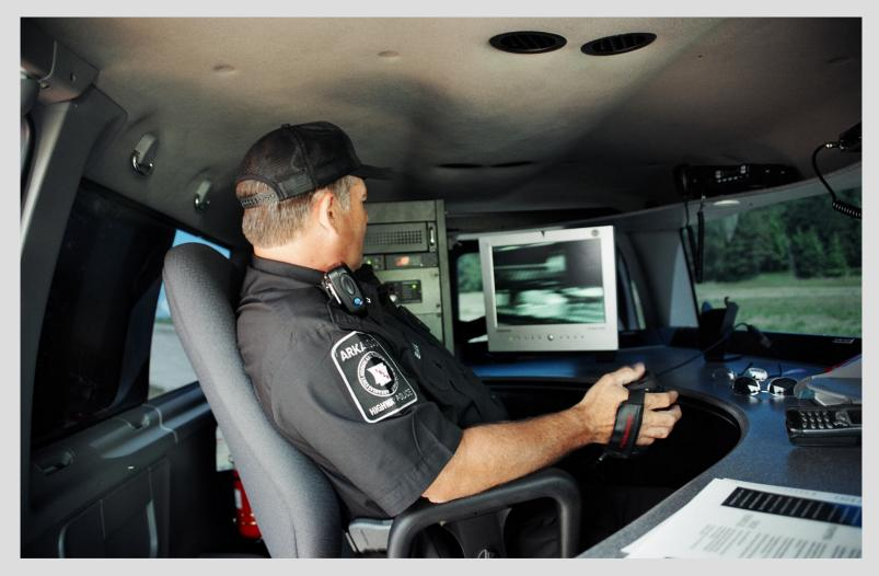
If the Brake is working it is generating heat the Flir is looking for Brakes not generating heat.
